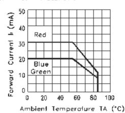
Fig.3 FORWARD CURRENT DERATING CURVE
