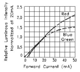
Fig.4 RELATIVE LUMINOUS INTENSITY VS. FORWARD CURRENT
