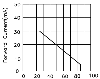
Ambient Temperature T_A (°C) FORWARD CURRENT DERATING CURVE
