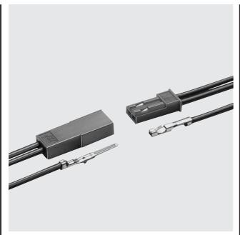
The RCY connector is a compact, 2.5 mm pitch wire-to-wire connector for use with a variety of circuits, from signal circuits to power supply circuits, in electrical equipment which is becoming more and more compact. The employment of a free spring contact method ensures stable contact performance, and superb working efficiency of insertion and removal.
