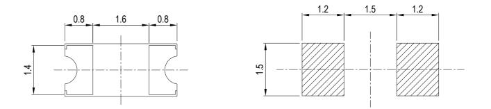
**Note:** The tolerances unless mentioned is  $\pm 0.1$ mm, Unit = mm
