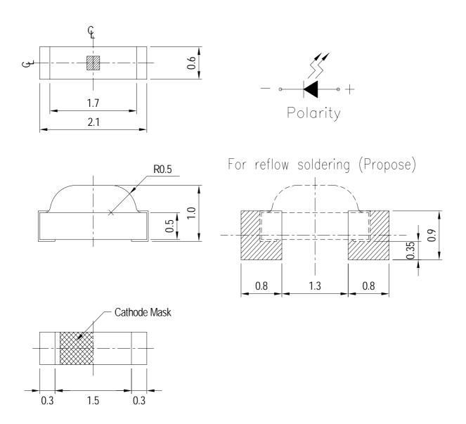
**Note:** The tolerances unless mentioned is  $\pm 0.1$  mm, Unit = mm
