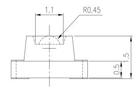
For reflow soldering (propose)
