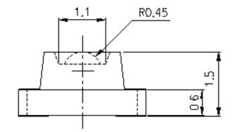
For reflow soldering (propose)
