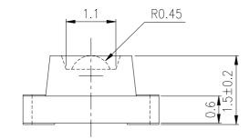
For reflow soldering (propose)
