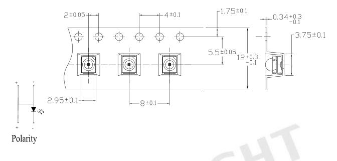
**Note :** Tolerances unless dimension is  $\pm 0.1$  mm, Unit = mm
