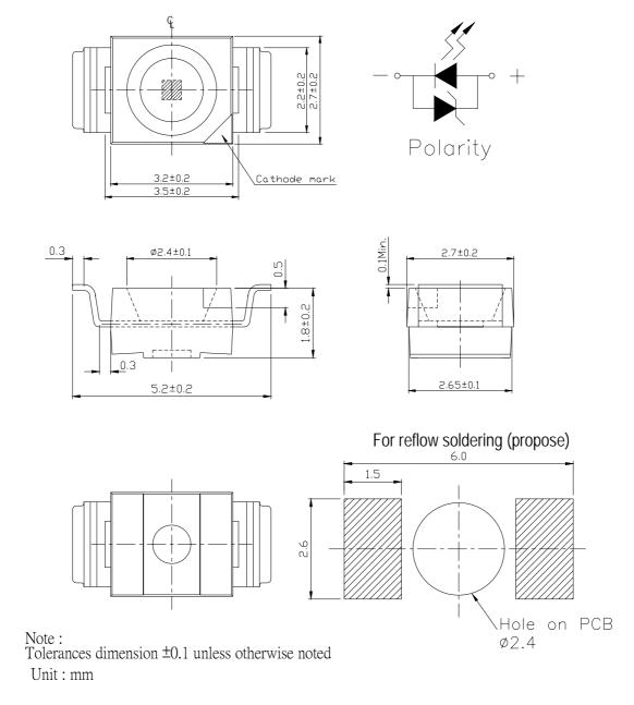
Notes: .All dimensions are in millimeters ,Unit = mm
