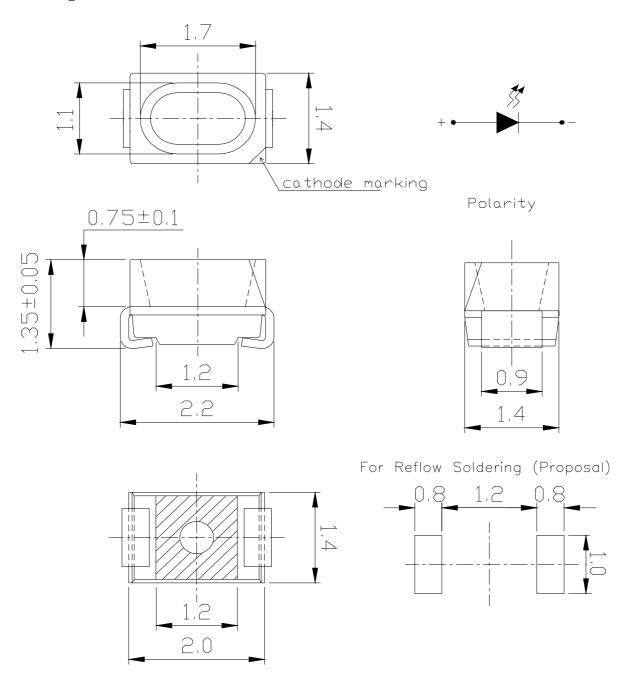
Notes: Tolerance of Dimension:  $\pm 0.1$ mm. Unit = mm
