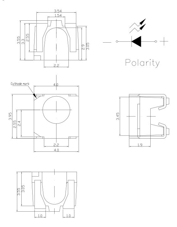
**Note:** The tolerances unless mentioned is  $\pm 0.1$ mm, Unit = mm
