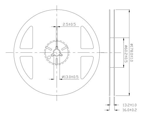
**Note:** Tolerance unless mentioned is  $\pm 0.1$ mm, unit = mm.
