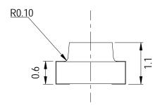
For reflow soldering (propose)
