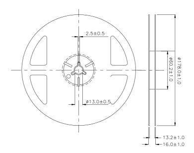
**Note:** Tolerances Unless Dimension is  $\pm 0.1$ mm, Unit = mm
