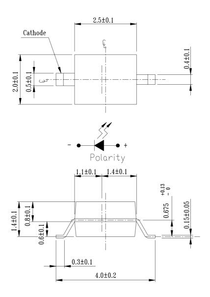
**Note:** Tolerances Unless Dimension is  $\pm 0.1$ mm, Unit = mm
