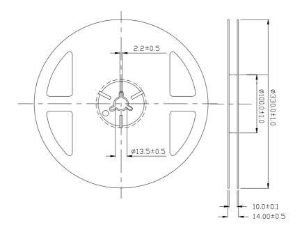
**Note:** The tolerances unless mentioned is  $\pm 0.1$ mm, Unit = mm
