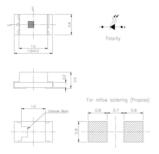
**Note:** Tolerances Unless Dimension is  $\pm 0.1$ mm, Unit = mm
