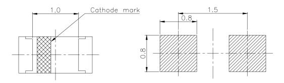
**Note:** The tolerances unless mentioned are  $\pm 0.1$ , unit = mm.
