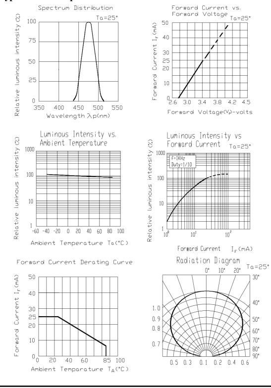
**Typical Electro-Optical Characteristics Curves**
