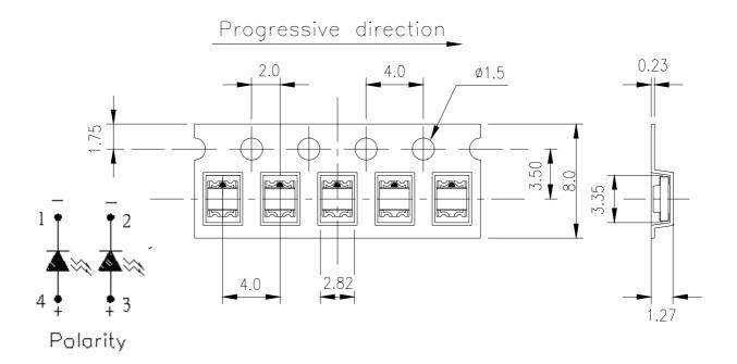
**Note:** Tolerances Unless Dimension ±0.1mm, Unit = mm
