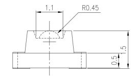
For reflow soldering (propose)
