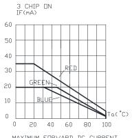
MAXIMUM FORWARD DC CURRENT VS, AMBIENT TEMPERATURE.
