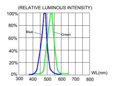
FIG.4 RELATIVE LUMINOUS INTENSITY VS. WAVELENGTH.
