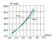
FIG.1 FORWARD CURRENT VS. FORWARD VOLTAGE.
