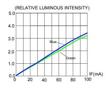
FIG.2 RELATIVE LUMINOUS INTENSITY VS. FORWARD CURRENT
